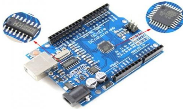
Figure 2: Arduino UNO SMD R3 Microcontroller Board
